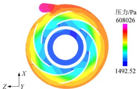
图 17 1000 L/h 离心泵轴向中间截面压力云图 Fig. 17 Pressure nephogram of pump in 1000 L/h of middle axial area
